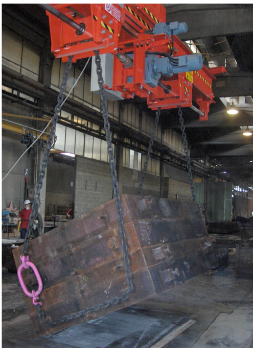
Manipulator for flask 20 ton
