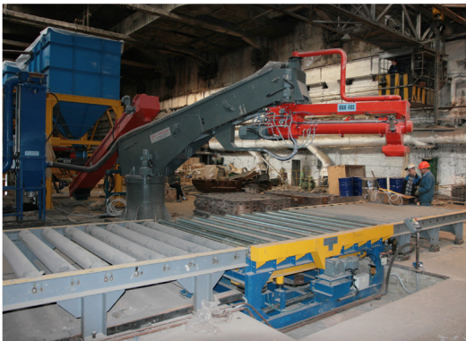
Articulated Mixer 40 ton/h and compaction table
