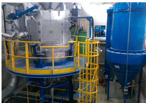
Sand Thermal Regeneration Plant - Simplex 1000 E
