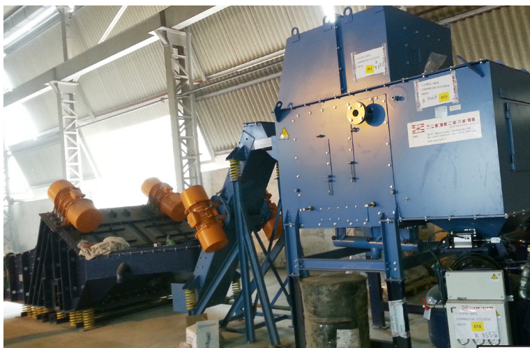
Shake-out and Mechanical Reclamation 8 ton/h
