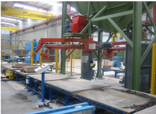
Mixer 20 ton/h and compaction table
