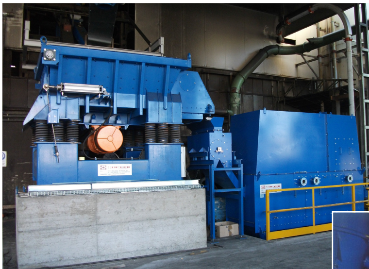
Mechanical Reclamation 20 ton/h
