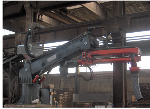
Mixer 30 ton/h with adjustable sand outlet level
