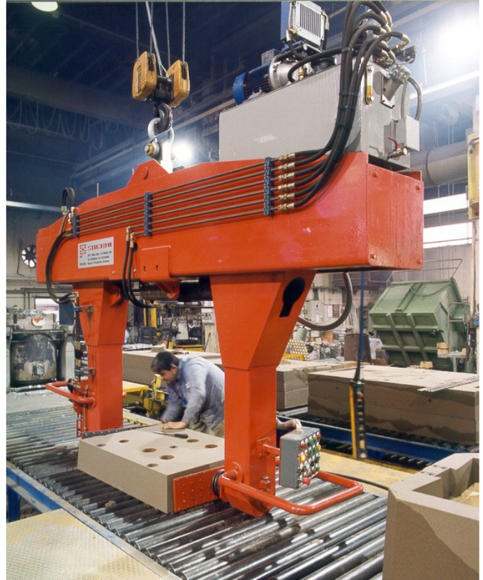
Manipulator for mould 3 ton
