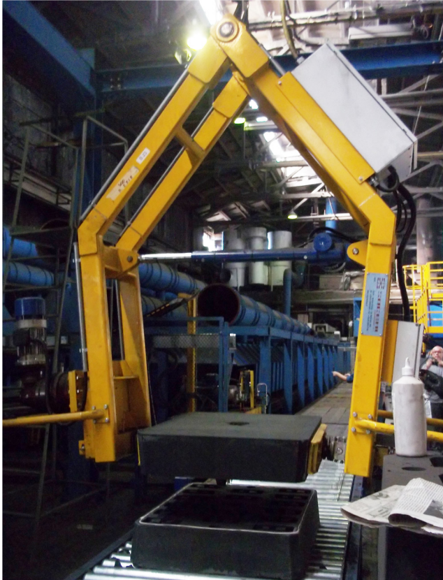
Manipulator for mould
