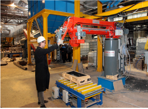
Pivoting Mixer 10 ton/h and compaction table
