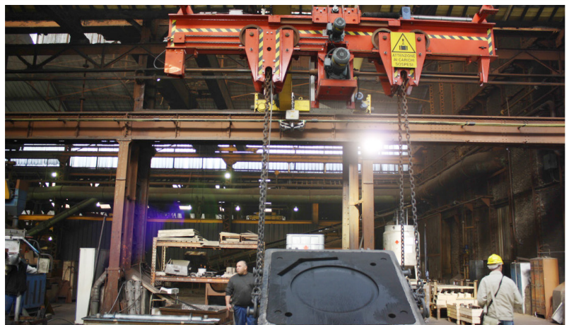
Manipulator for flask 10 ton
