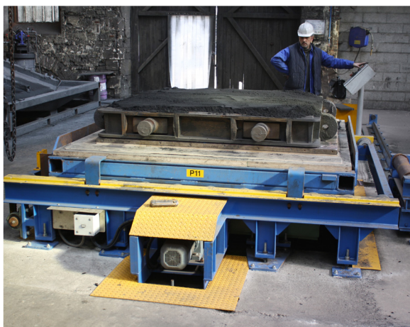
Stripping station for flask of 10 tons loading
