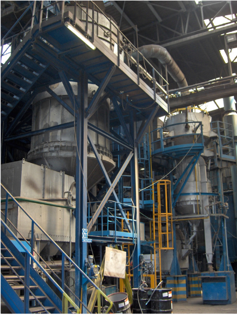
Thermal reclamation 5 ton/h and 2 t/h
